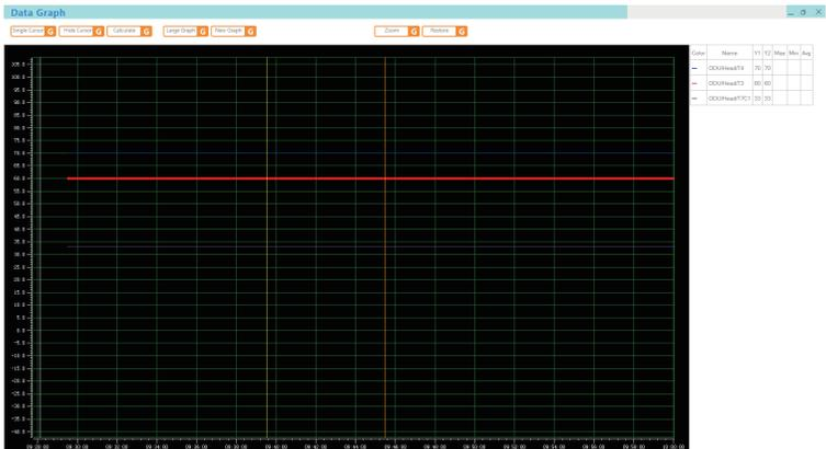
**Large Graph G** - Display the maximum range of the graph, such as all the data for 3 days when the M-DT has been operating for 3 days.
