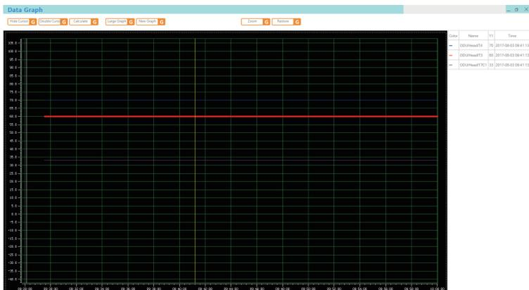
A yellow cross will appear on the interface. Use the mouse to drag the cursor, and once the mouse is released, the right side will be refreshed to show the parameters at where the cursor is.
