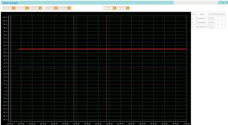
There are two cursors on the interface: yellow and ochre. Use the mouse to drag the cursor, and once the mouse is released, the right side will be refreshed to show the parameters at where the cursor is.
